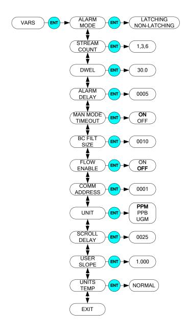
Figure 7-3: Front Panel Menu Diagram (Page 2)
